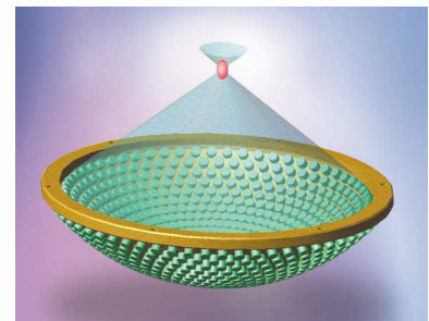
Piezo transducer surface with its mosaic design.
